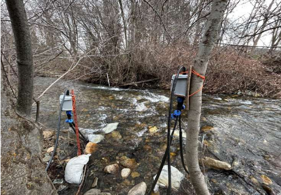
Picture 5. French Creek downstream array. J-boxes in foreground attached to t-post and tree.
