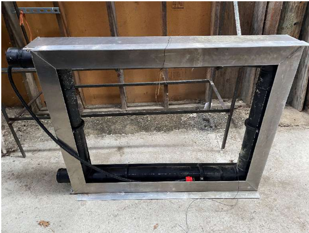
Picture 2. HDPE antenna operated at Scott River weir.
