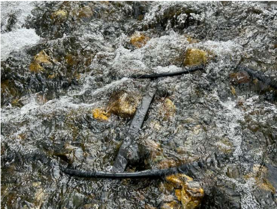
Picture 6. Flexible antenna lying flat on streambed at French Creek downstream array.
