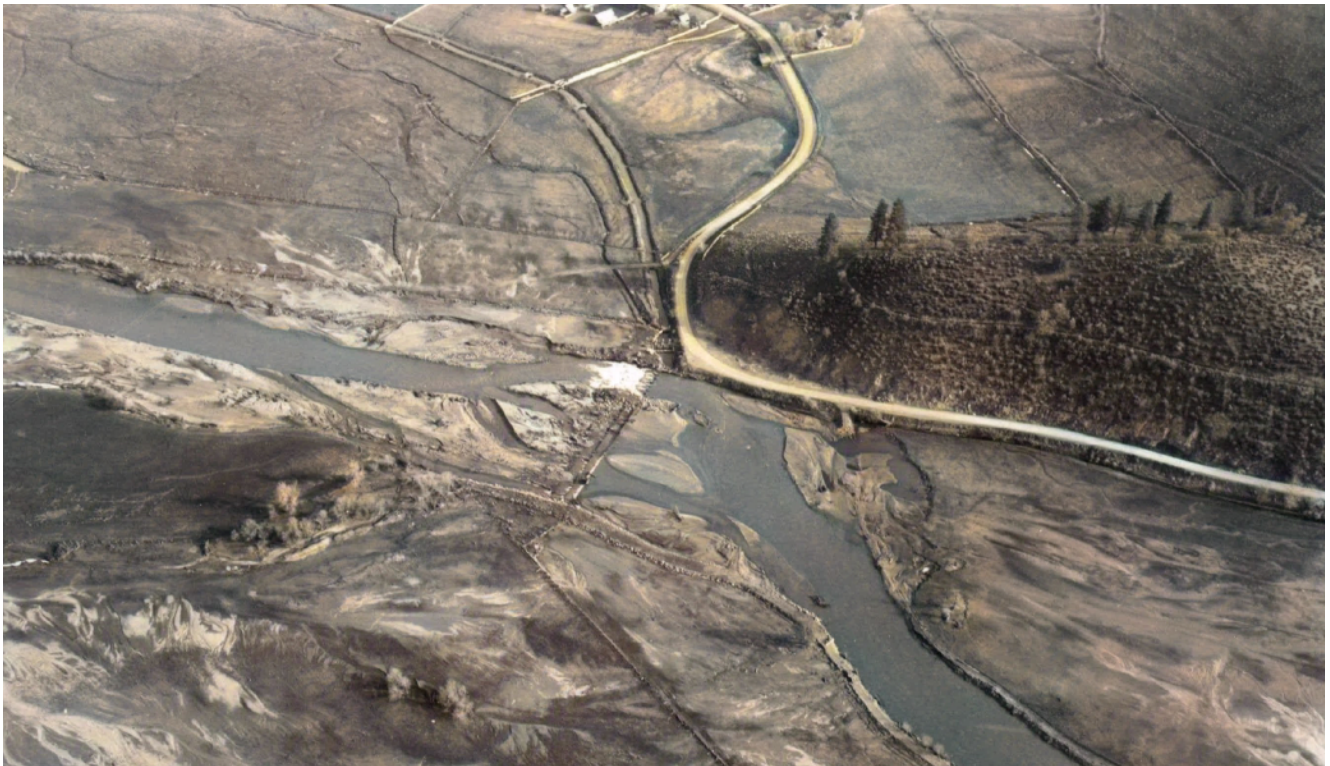
Scott River at Young's Point and Scott Valley Irrigation District Point after December 1964 flood. This flood was the largest on record with a peak discharge of 54,600 cubic feet per second.
