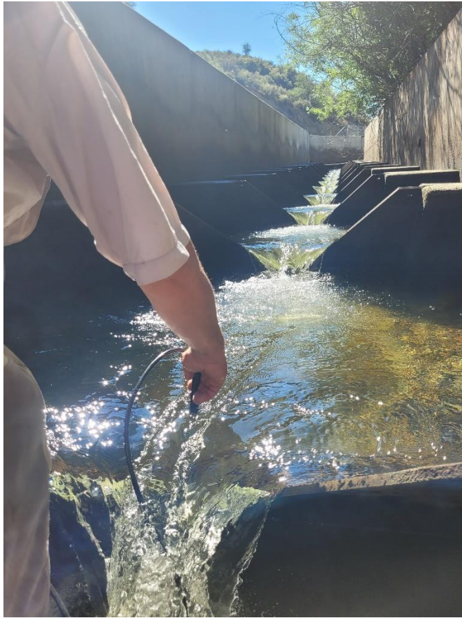
Photo 10. Measuring velocity in the V notch of baffle 1 at 1.85 cfs.
