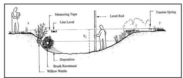
Measuring a stream cross section
