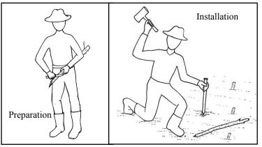
Note: Posts (3 to 6-inch diameter) are prepared and installed very similar to poles. However, power augers are used more often to create the holes.
