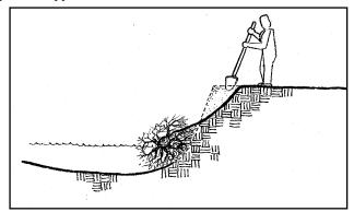
Option 2: In areas of higher stress, as can be found along the outer bank of a turn, anchor the revetment over a stone toe with soil anchors. In the detail shown below, live poles are also specified.
