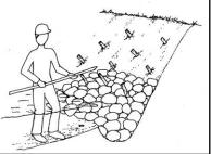
The above figure shows a stone toe and live poles. The stone is keyed into the bed below an anticipated scour depth. Live poles can be installed with the aid of a waterjet stinger.
