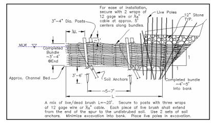
Option 2: In areas where a longer spur is needed, overlap a mixture of live and dead material by a minimum of  $\frac{1}{2}$  the length of the brush. Secure the material together with 2 wraps of wire or cable at approximate 5 feet centers along the bundle.
