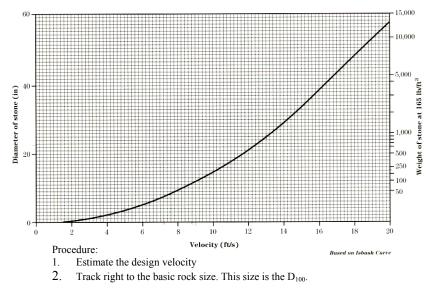
**Gradation:** The gradation of stones in riprap affects its resistance to erosion. Specifications typically include two limiting gradation curves. USACE EM 1110-2-1601 (1991) contains standardized gradations for riprap placement in the dry, low turbulence zones. One is provided below.
